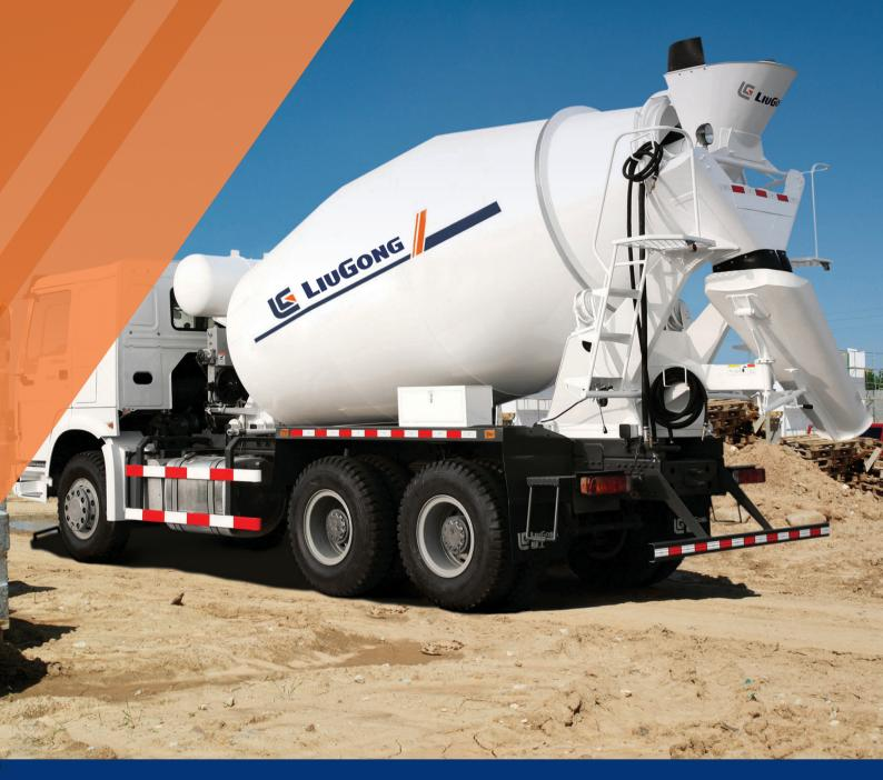
Drum Geometrical Volume Drum Agitating Capacity Concrete Charge Speed Concrete Discharge Speed Drum Remnant Ratio Drum Inclined Angle Water Reservoir Capacity Water Supply Type 17.2 m<sup>3</sup> 10 m<sup>3</sup> ≥ 3 m<sup>3</sup>/min ≥ 2.7 m<sup>3</sup>/min < 0.5% 12.5° 450 L Pneumatic Pressure
